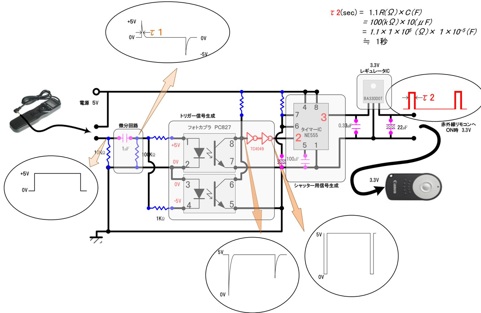
$$\begin{aligned} \tau 2(\text{sec}) &= 1.1R(\Omega) \times C(F) \\ &= 100(k\Omega) \times 10(\mu F) \\ &= 1.1 \times 1 \times 10^5 (\Omega) \times 1 \times 10^{-5} (F) \\ &\approx 1 \text{秒} \end{aligned}$$
